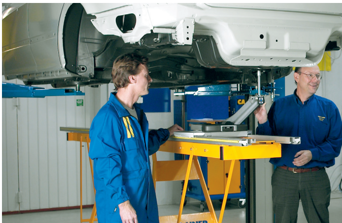
M802 with Measuring Bridge and Car-O-Tronic Vision2 X3
