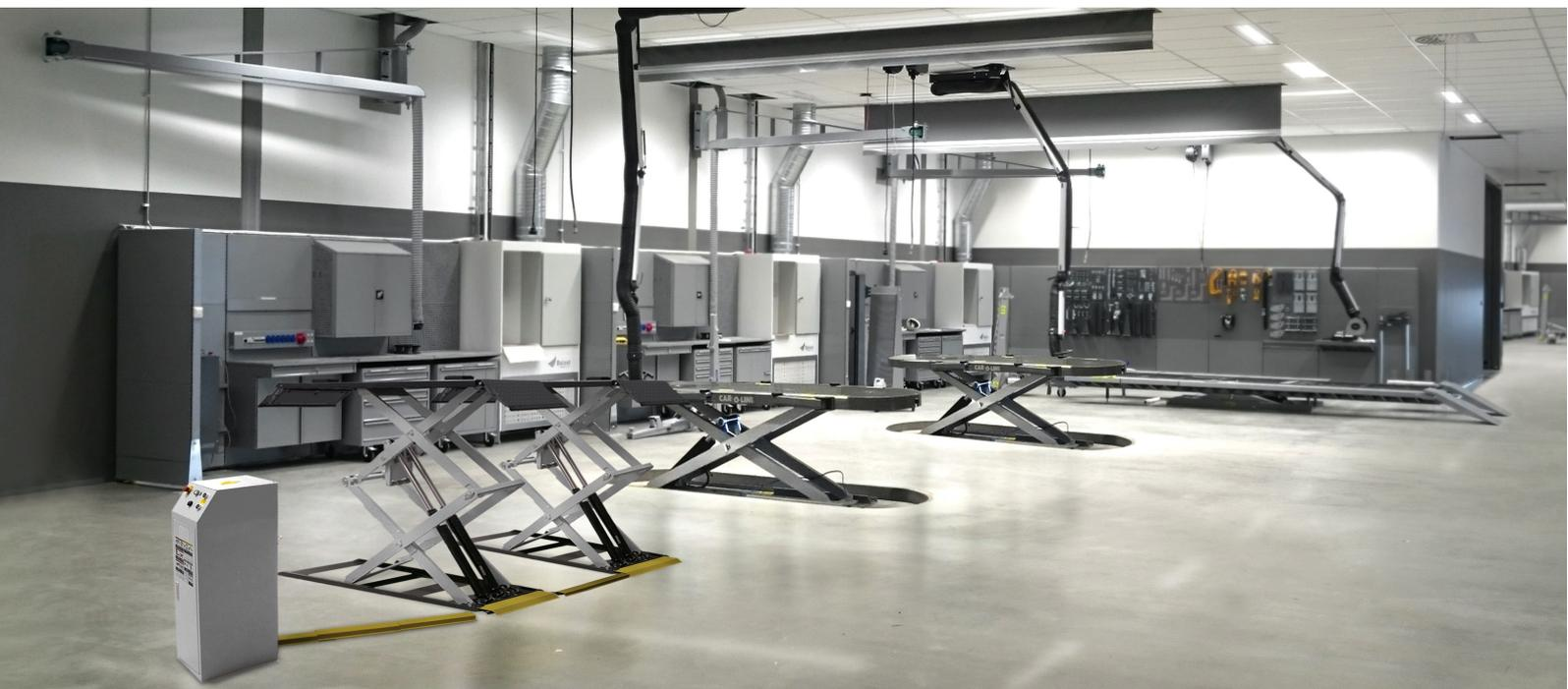
THE CDS 35 DOUBLE SCISSOR LIFT HAS A PROFILE TO DRIVE/ROLL ANY VEHICLE OVER IT FOR FAST REPAIR WORK.
