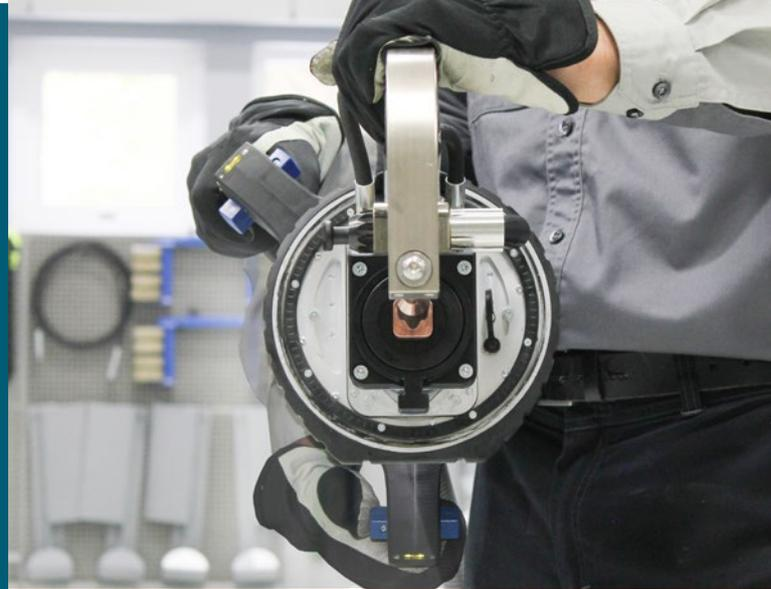
The handle swivels 355° on two axes. Just press the quick-release button and turn the handle to an optimal working position for superior handling.
